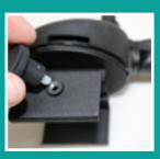
4. Fit the control unit holding screw into place on the side of the control unit bracket, by screwing into place. This will only take a small amount of turning. \*\*If the control unit will not slide into the control unit bracket, unscrew the holding screw slightly. When the control unit is positioned in the bracket, tighten the holding screw to keep the control unit in place during operation.
